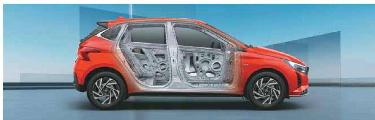
Strong body structure (with AHSS and HSS)
